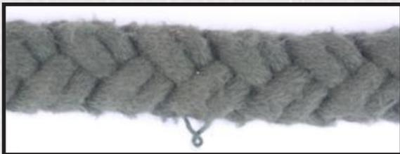
**Picture 2: Hooked yarn under 25mm**
